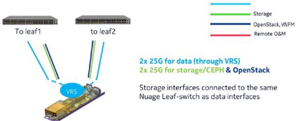
Figure 3.54 : Connectivity from compute servers to the leaf switches
