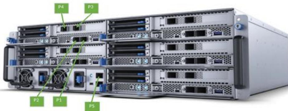
Figure 3.84 : OE19 Chassis networking ports
